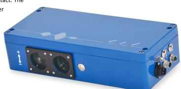
The measurement object is imaged onto the CCD sensor by an objective. The CCD sensor is operated as an optical grid (no image acquisition). The measurement object is illuminated by an integrated light source (LED). When the object is moved, a signal frequency is generated due to the grid modulation. This frequency is proportional to the velocity at which the object is moving. The device measures the signal frequency and converts it into a velocity value. Several loop control circuits enable
